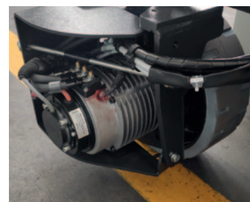
AC electric motor. 90° wheel steering.
